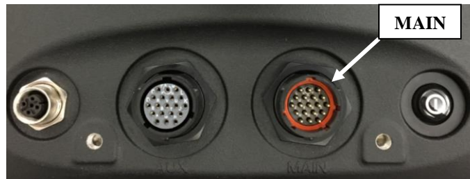
Figure 3. Display cable connection
