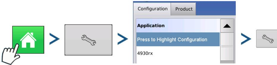
Press: Home button > Setup (wrench) button > select specific configuration > Setup (wrench) button
