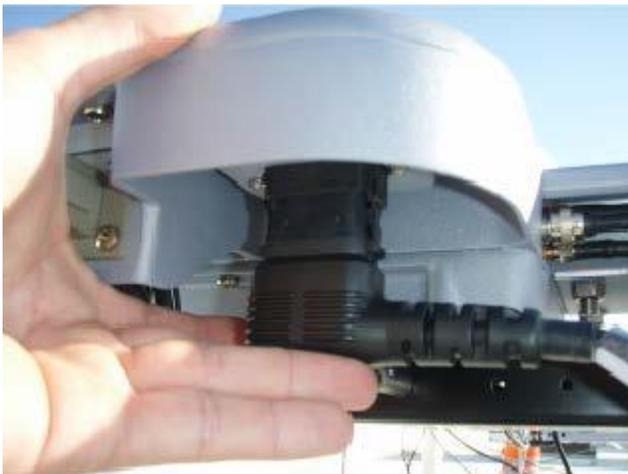
4. Insert USB into the USB slot on the Aux Harness
