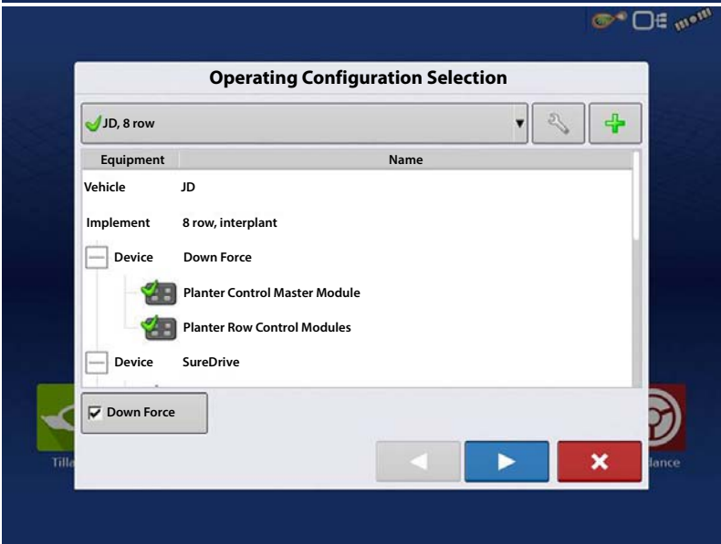
Image 4 - How the Field Select Wizard should appear when all RCM modules have been found on the CAN Bus, properly indexed, and properly assigned to each of the rows.
