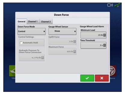
**Control mode**—as the planter travels across the field and encounters varying soil conditions (soil types, compaction zones, levels of debris) the display makes adjustments to the down force actuators on the row units, according to the operator's settings, to maintain the correct seed placement in the soil.
