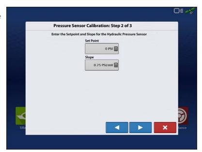
**Pressure to Force**—Enter the specific pressure to force conversion ratio for the planters parallel linkage arm. Press the . Pressure Sensor Calibration is complete.
