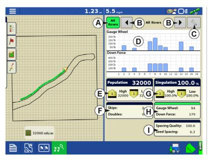
Screen will show Gauge Wheel readings and Down Force across the row sections of the planter.
